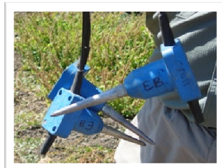
Geophones for soft ground types (Type I)
