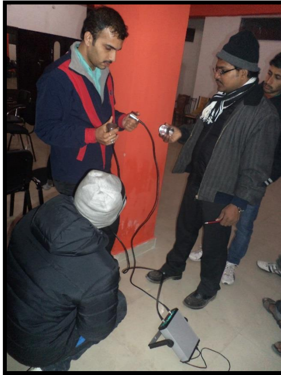
Figure 74: Ultrasonic Pulse Velocity Method (Kangra, 17th December 2013)
