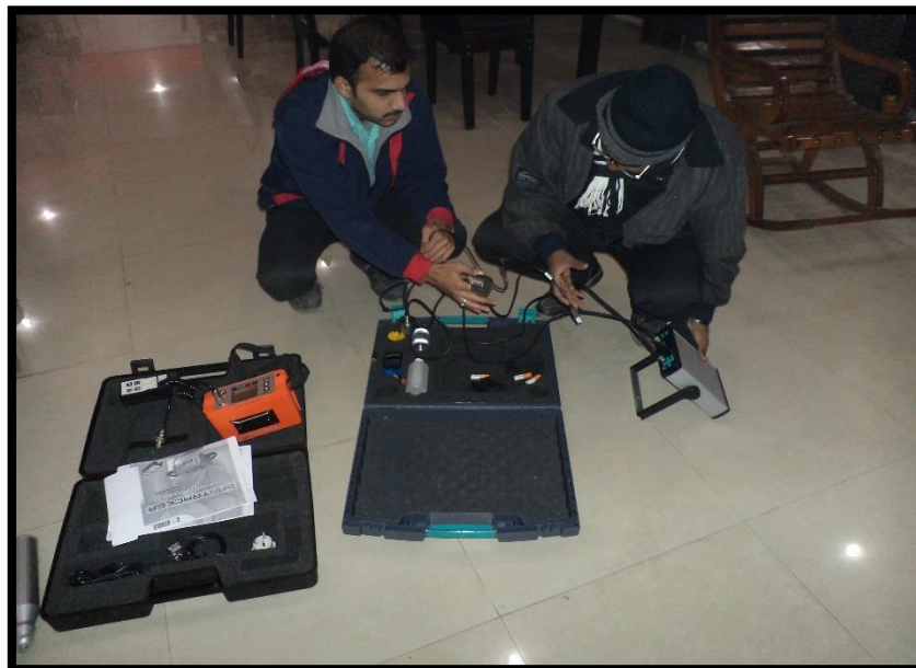
Figure 75: Preparation of instrument before Ultrasonic Pulse Velocity Method (Kangra, 17th December 2013)
