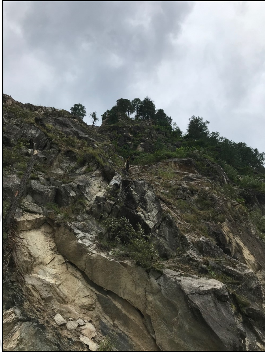
Fig. 4: Highly jointed rock mass exposed along cut slopes in Nigulsari landslide area, Kinnaur District
