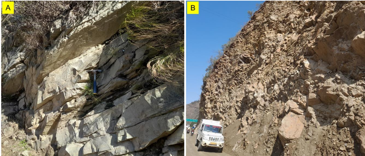
Photo 9. The hillward dipping dark grey to grey, hard and massive quartzites exposed at the level of NH-154A.
