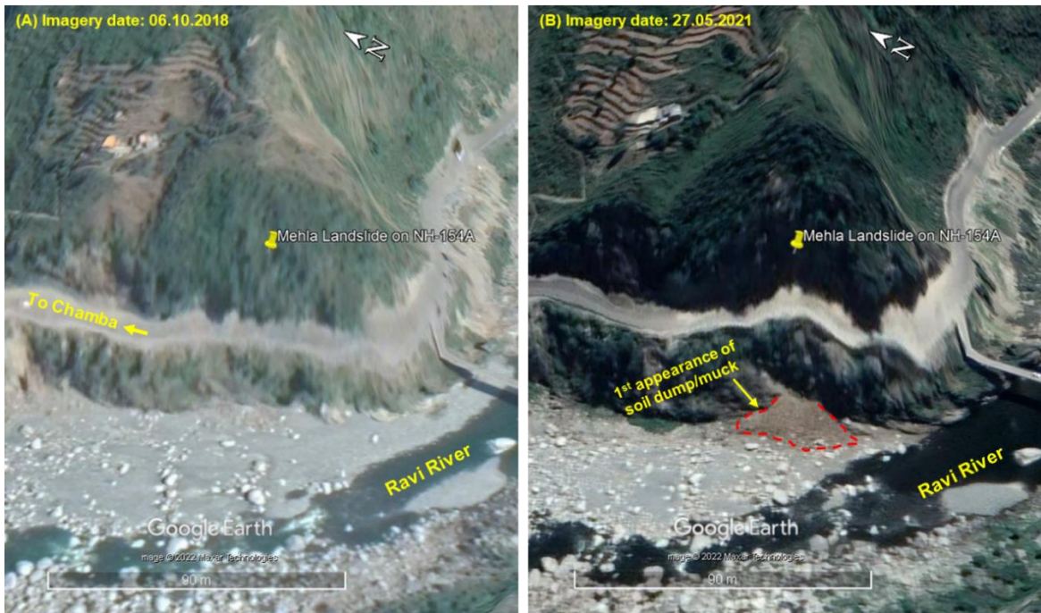
Photo 4. Temporal Google Earth images for the Mehla landslide; (A) Normal slope conditions prior to 06.10.2018, (B) Slight hillward curvature of the road and sudden appearance of soil dump/muck downslope of road.
