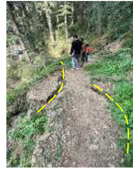
Figure 8 (g) Titling of trees and ground cracks observed at crown
