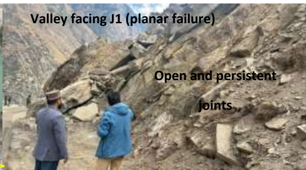
Figure 25(e) Open and persistent Valley facing joints
