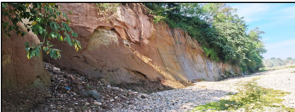
Fig. 13: Quaternary deposits as observed along open joints/fractures in weathered rock mass, as observed along right bank of Sukar Khad .
