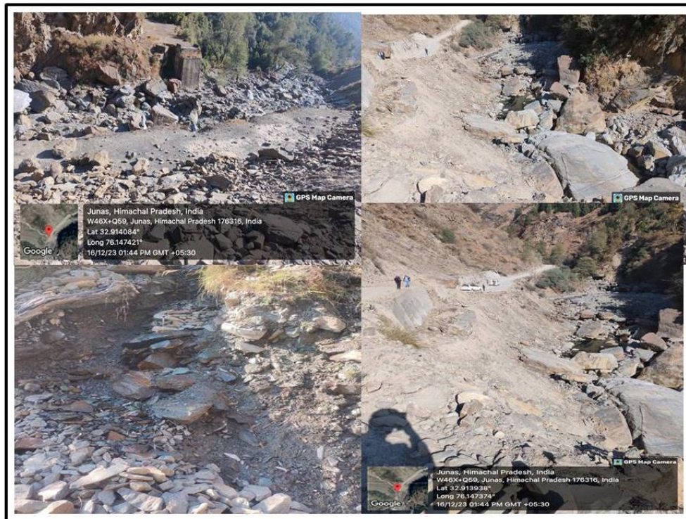
Fig.48 a) Shows the damaged part of the road and retaining wall along the Tarela-Boundary Mangli Road slide zones b & d) indicated large chunk of slates and boulders which can be used to diver the river channel and slope angle of the slide zone c) shows the moisture content and irregular stones which have been broken from the in situ rock.
