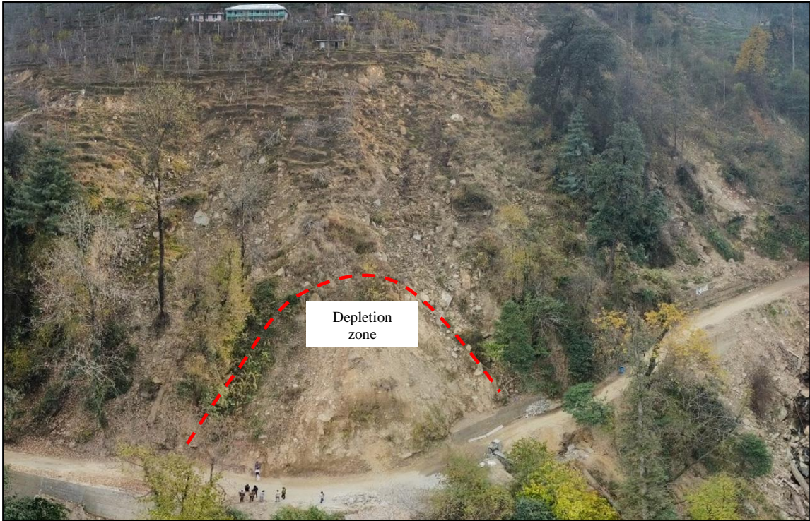
Fig. 56. Field photograph showing depletion zone and threatened apple orchards
