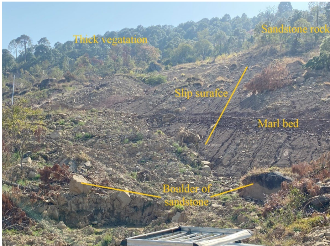
Fig. 12 Highly fractured sandstone bed moved along the slip surface of the marl bed.
