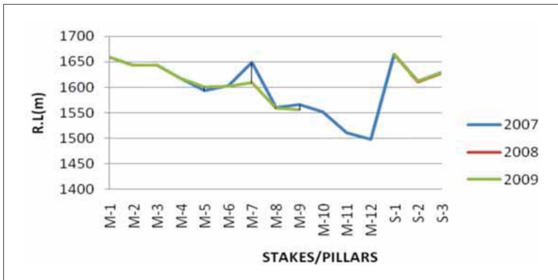
Fig. 3.23. Ground displacement curve obtained using monitoring of stakes/pillars at Surbee landslide zone.
