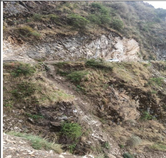
Fig. 3 Steep slope on hill and valley side. Valley side has thin layer of debris underlain by jointed rock mass
