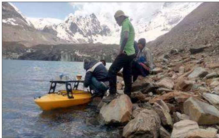
Photo -1 : Bathymetry survey on Geepang Gath Lake using RCV boat fitted with echo-sounder and GPS
